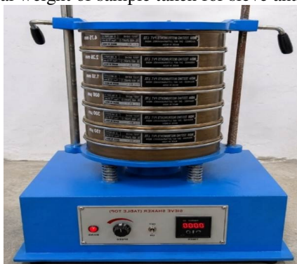
Fig. 7 : Particle size distribution analysis using a sieve shaker
