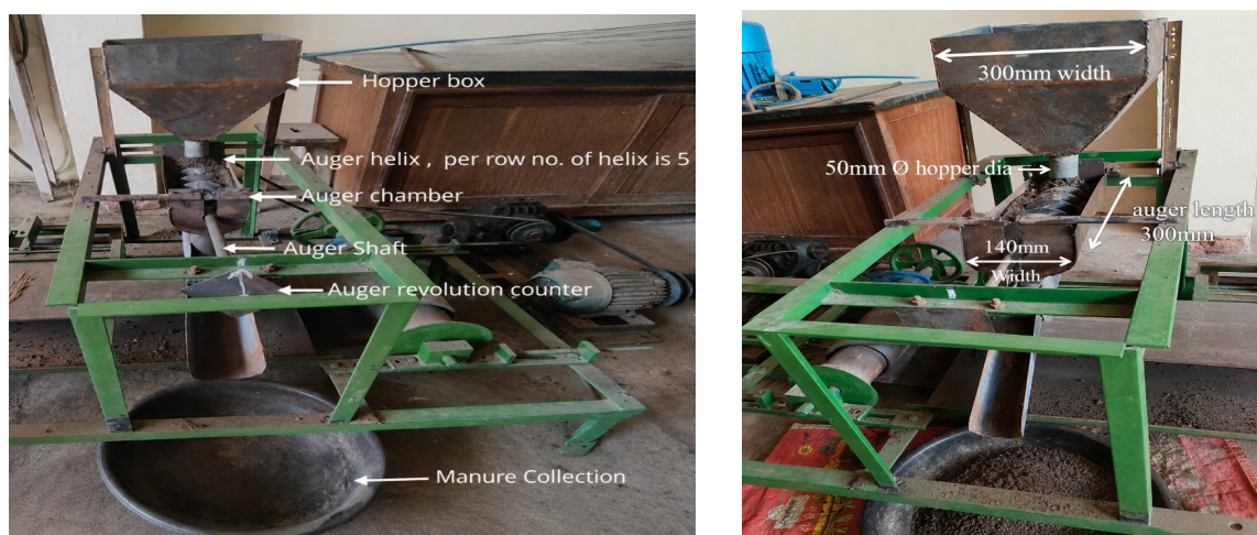
Fig. 10 : Prototype Machine for Laboratory Evaluation Manure Discharge Performance
