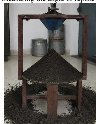
Fig. 8.1 : Angle of repose measurement of organic manure
