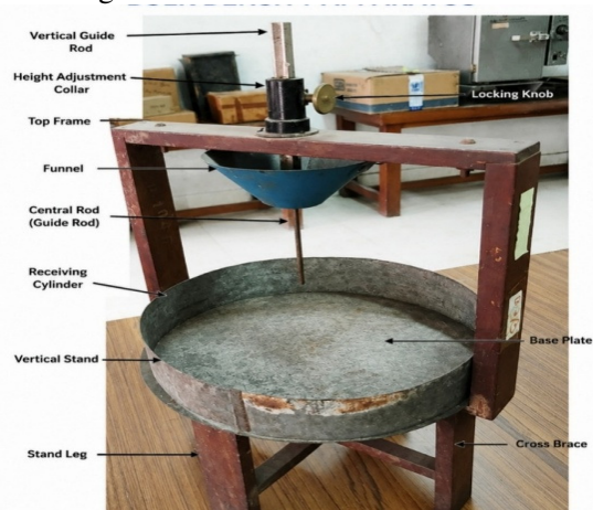
Fig. 8 : Measuring the angle of repose apparatus
